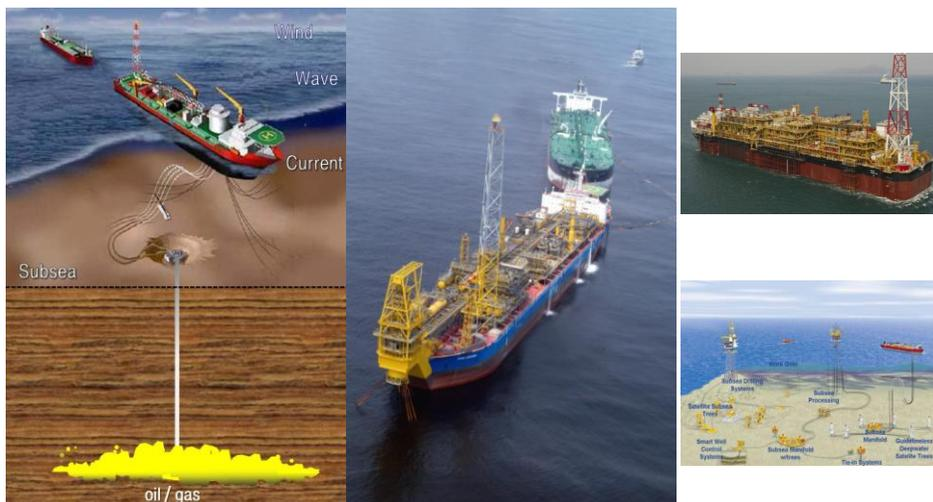
Vessel (hull), topsides (process facility), mooring, umbilicals/risers/flowlines, subsea, and export system
