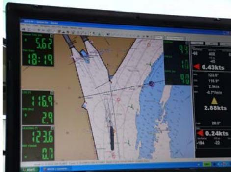
Figure 8. Ultra large container carrier approaching the Berendrecht Lock, Port of Antwerp, Belgium, from the riverside, assisted by a portable pilot assistance system.
