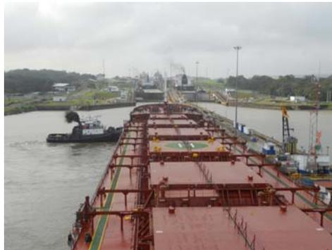
Figure 6. Bulk carrier pushed by tugs to the approach wall before entering Gatún Locks, Panama Canal.
