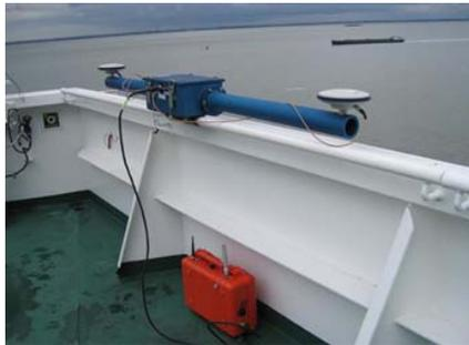
Figure 3: In situ measurement of vessel motion
