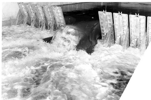
Fig. 5.3 : Flow conditions during raising of a bottom-hinged flap gate just before the gate breaks the nappe
